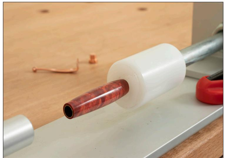
Once in place hand press the cap and clip onto the barrel. Next, slowly press the parts together by pushing the handle lever toward the pen. This pushes the aluminum stop towards the UHMW stop. Continue this motion until the cap and clip is pressed up against the top of the barrel. Finish assembling the pen and check all the mechanisms to make sure they are working properly.
